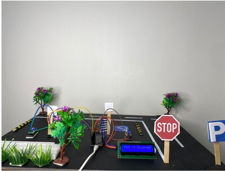
Fig. 2. The hardware implementation of our proposed IoT-based parking system
